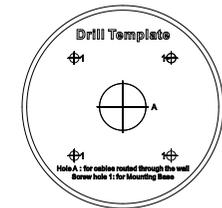
Figure 2-9 Drill Template of the Junction Box
